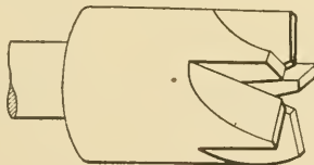
Fig. 249—A small running-down cutter that finds many uses
